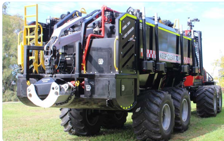
Forwarder crane tucks in for low profile
