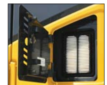
External air conditioner filter
